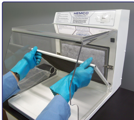
Replacement of pre-filter on Micro Flow II
